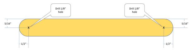
Why we do this: We need a place for our axels to pass through our transporter, so the wheels and axels don't fall off as the transporter moves. This is what is known as a fixed axel design and does not allow for steering to the right or the left.
